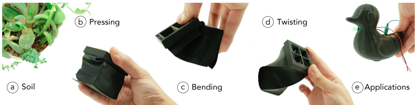
Figure 1: When pressure is applied to the cathode of an SMFC, its output voltage varies with the force. As a result, using soil as the core material (a), we can create a tangible interface that responds to (b) pressing, (c) bending, and (d) twisting, opening new design space for bio-based design and (e) applications.
